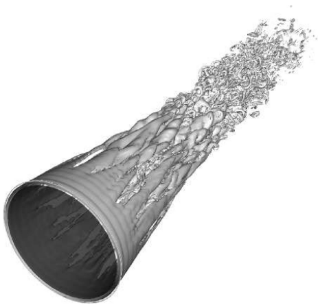
Fig. 9 Instantaneous perspective view of |W_{ik}|=5 for one-half-cylinder case: Re_D = 1 \times 10^5 and M = 2.46 .
